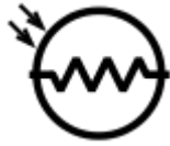
Fig 4.1 The symbol for a photoresistor
