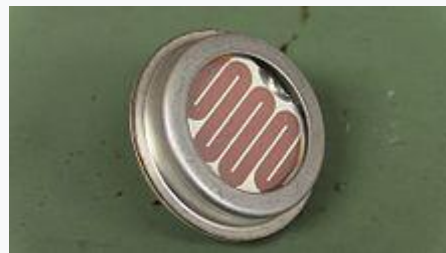
Fig 4.3. Large CdS Photocell from a street light.
