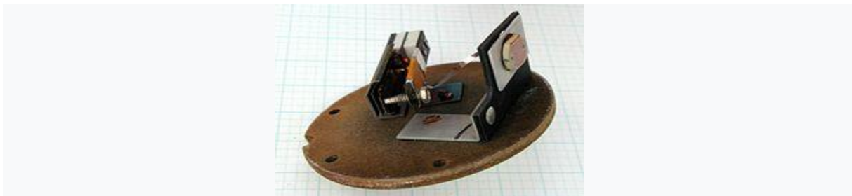
Fig 4.5. The internal components of a photoelectric control
